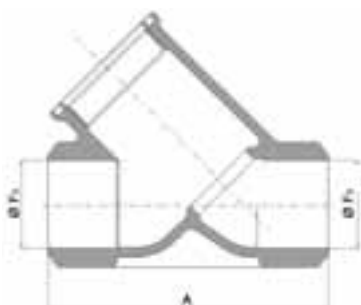
Valve with butt weld connection for ISO 4200 pipe Welding ends complying with ISO 6761
